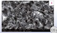
Fig. 4 Hybrid ceramic surface after hydrofluoric acid etching for 120 seconds
