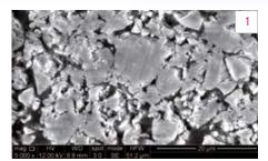
Fig. 1 Control group: unetched hybrid ceramic surface
