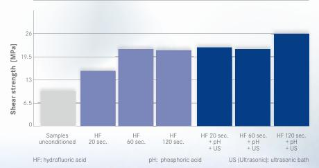
**Graph:** Shear bond strength of Bifix QM luting composite (VOCO GmbH) to VITA ENAMIC (VITA Zahnfabrik) after pretreatment of VITA ENAMIC with different conditioning types/protocols.
