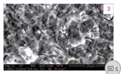
Fig. 3 Hybrid ceramic surface after hydrofluoric acid etching for 60 seconds
