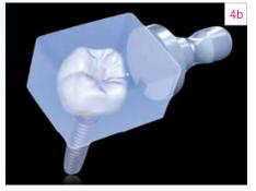
Fig. 4b ...and the milling preview prior to the CAM process.
