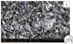
Fig. 2 Hybrid ceramic surface after hydrofluoric acid etching for 20 seconds
