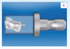
Fig. 8 In the grinding preview, the designs were placed optimally in the blank (the inlay for tooth 26 is shown).
